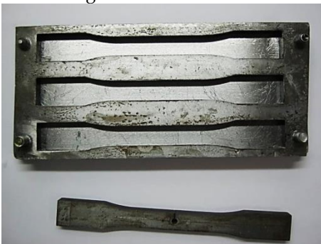
Fig. 5: Steel Mold and Dummy Steel Specimen
