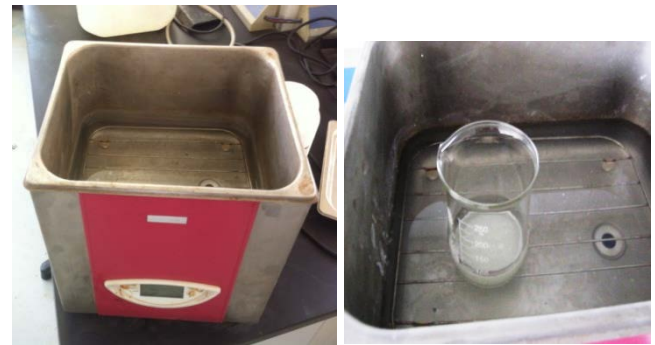
Fig. 2: Ultra-Sonication Bath and Alumina Specimen (FUNGILAB S.A)
