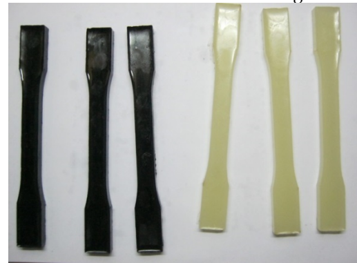
Fig. 6: 1wt% G and 1wt% Al 2 O 3 nanoparticle reinforced epoxy composite specimen.
